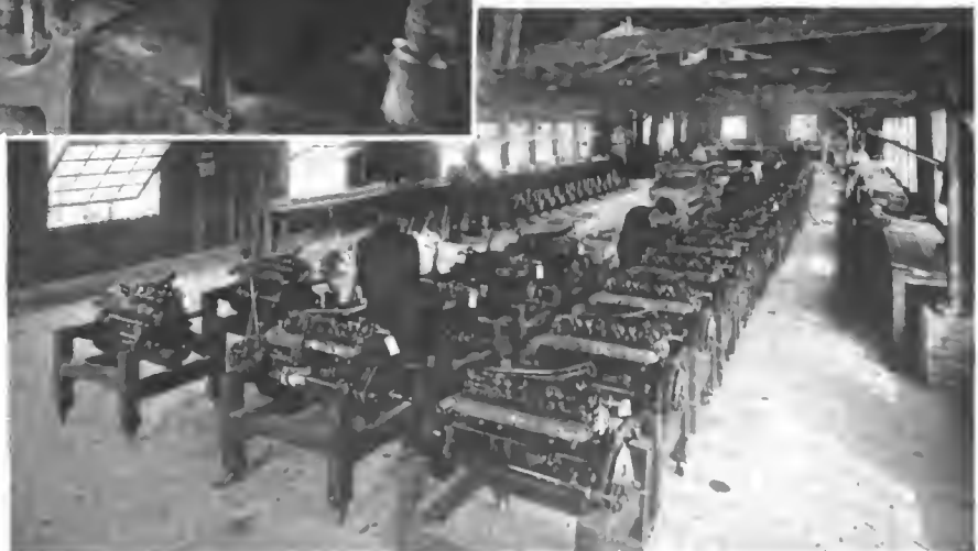
Above—Part of the engine testing room at the plant of the Liberty Motor Car Co., showing the type of testing blocks used and the cooling water connections employed for the test runs
